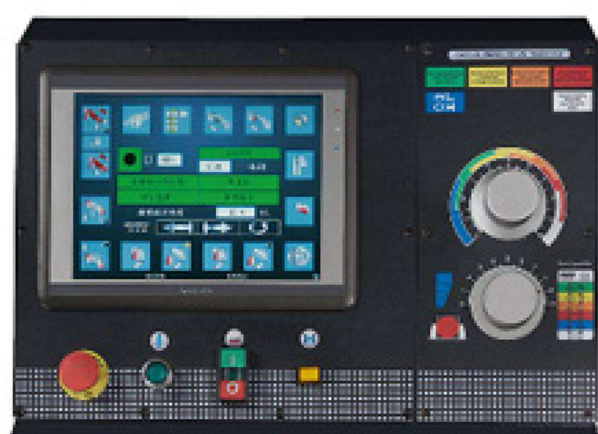
■ 3D HMI control panel.
