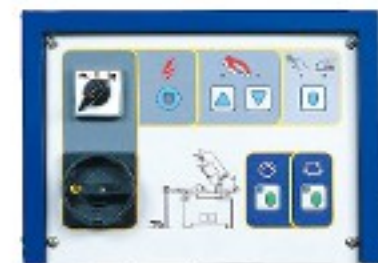
ELECTRONIC OPERATION CONTROL PANEL With lights for indicating or trouble-shooting problems.
