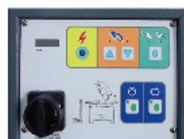
Variable speed with inverter.
