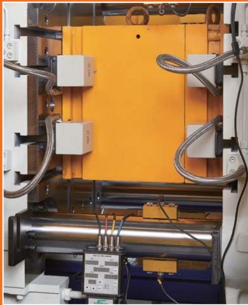
INSPECTION OF AVERAGE LOAD FOR CLAMPING FORCE 鎖模力平均負載檢測
