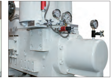
Shot velocity-controlled scale & pressure sensor. 射出速度控制刻度錶及壓力感測器
