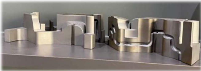
Material: SUS420J2 Hardness: HRC50±2
