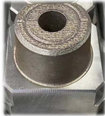
Material: M789(Corrax) Hardness: HRC48~50
