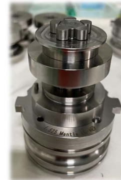
Material: SUS420J2 Hardness: HRC38~42
