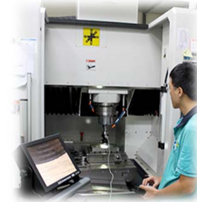
TOLTEC Contour Profiler On-Machine Inspection
